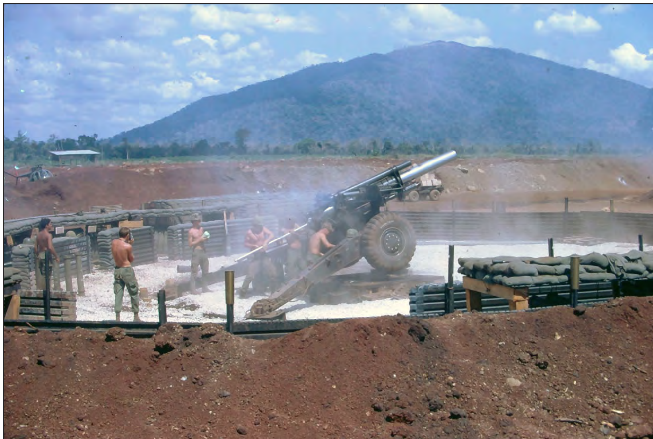
Preparing to fire a 155mm howitzer. Two crew members are ramming home the shell.
