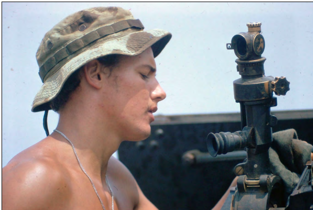
A gunner cleaning the sight on a 155mm howitzer. A spirit level used as part of the aiming mechanism is visible just below the sight.
