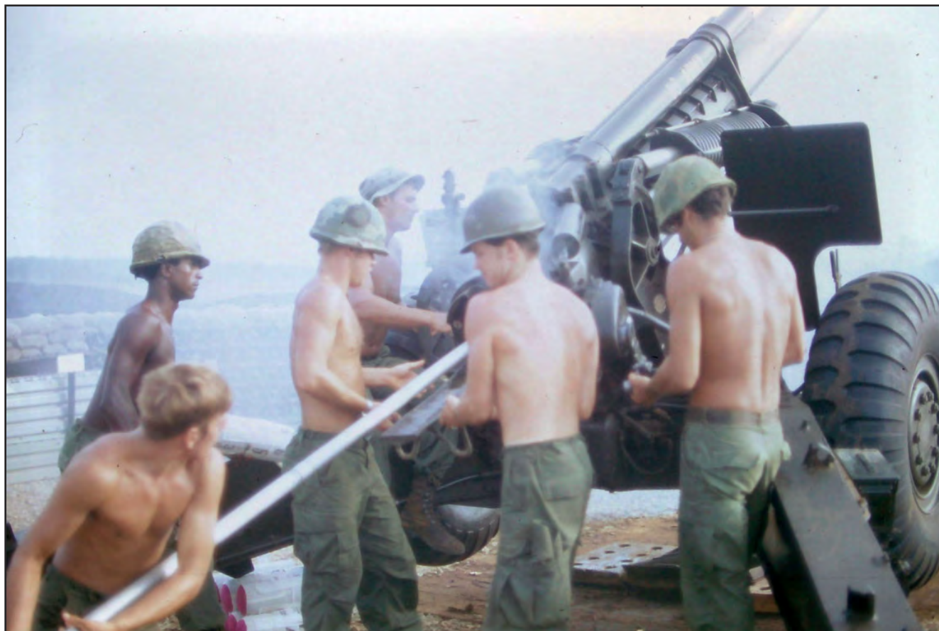
A sequence of four photographs showing the steps in the firing of a 155mm howitzer. In this first one, two men have carried a shell to the howitzer on a metal tray, and another crew member is using a long ramrod to seat the shell in the barrel. I remember taking this sequence deliberately to have a record of these separate actions.
