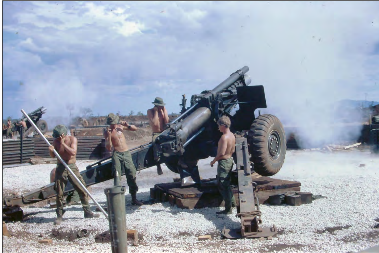
The moment of firing the howitzer. The barrel is in full recoil position.
