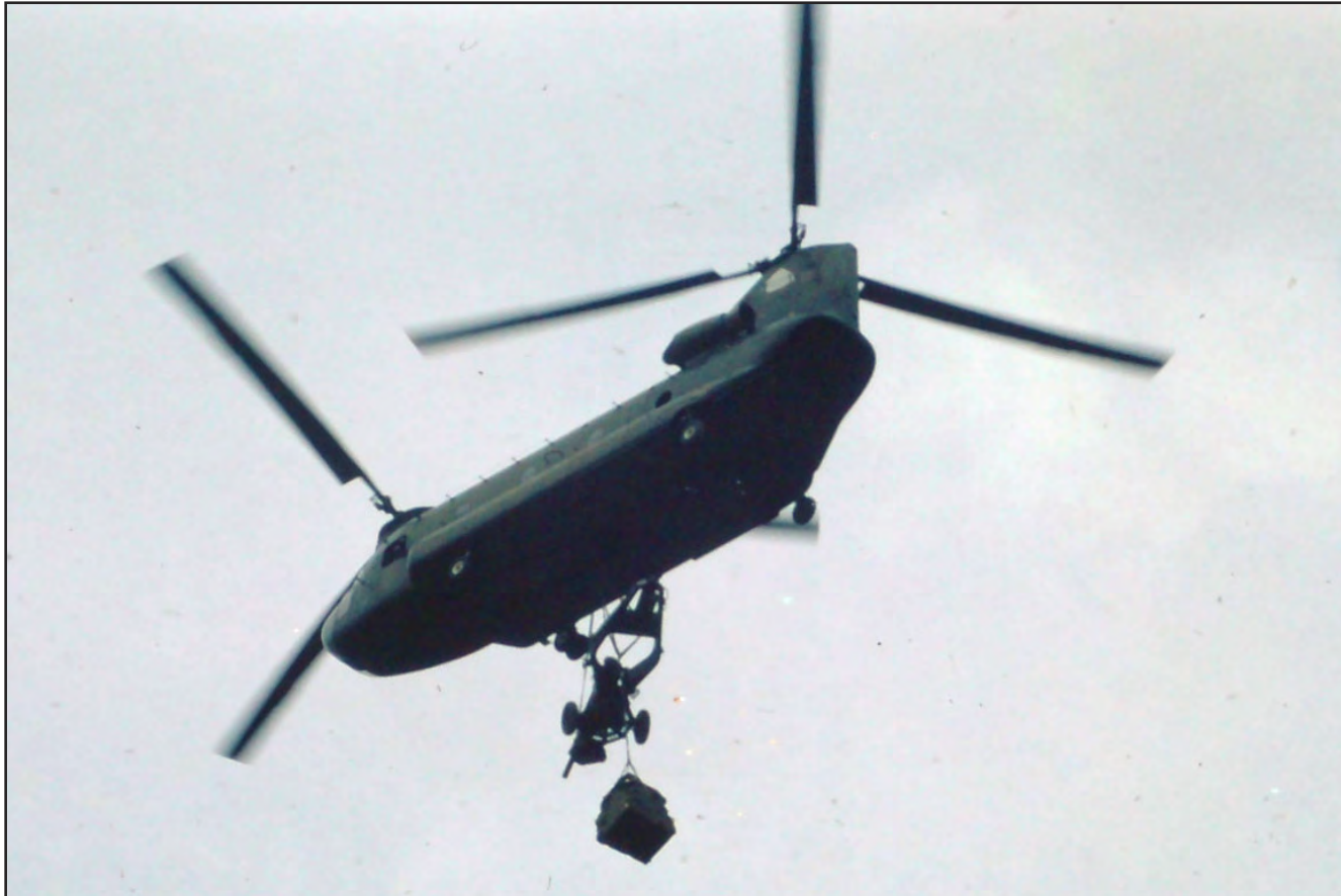
A helicopter carrying a 105mm howitzer and its ammunition load from our base to another field location.
