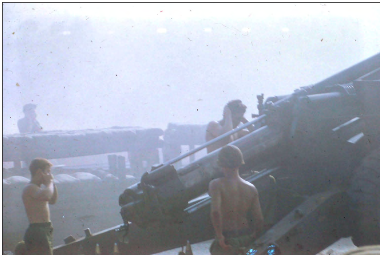
Another view of the full recoil position of the barrel. Smoke from this and other howitzers firing nearby dims the view in this photograph. More shells with fuzes attached may be seen in the bottom left, in front of the crewman on the far left.
