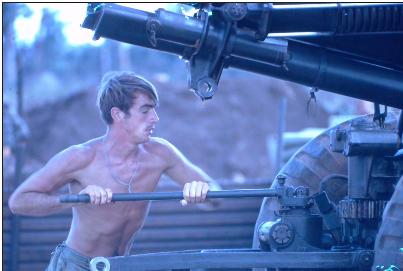
Jacking up the center pivot of the howitzer so that it could be moved to point to a new location.
