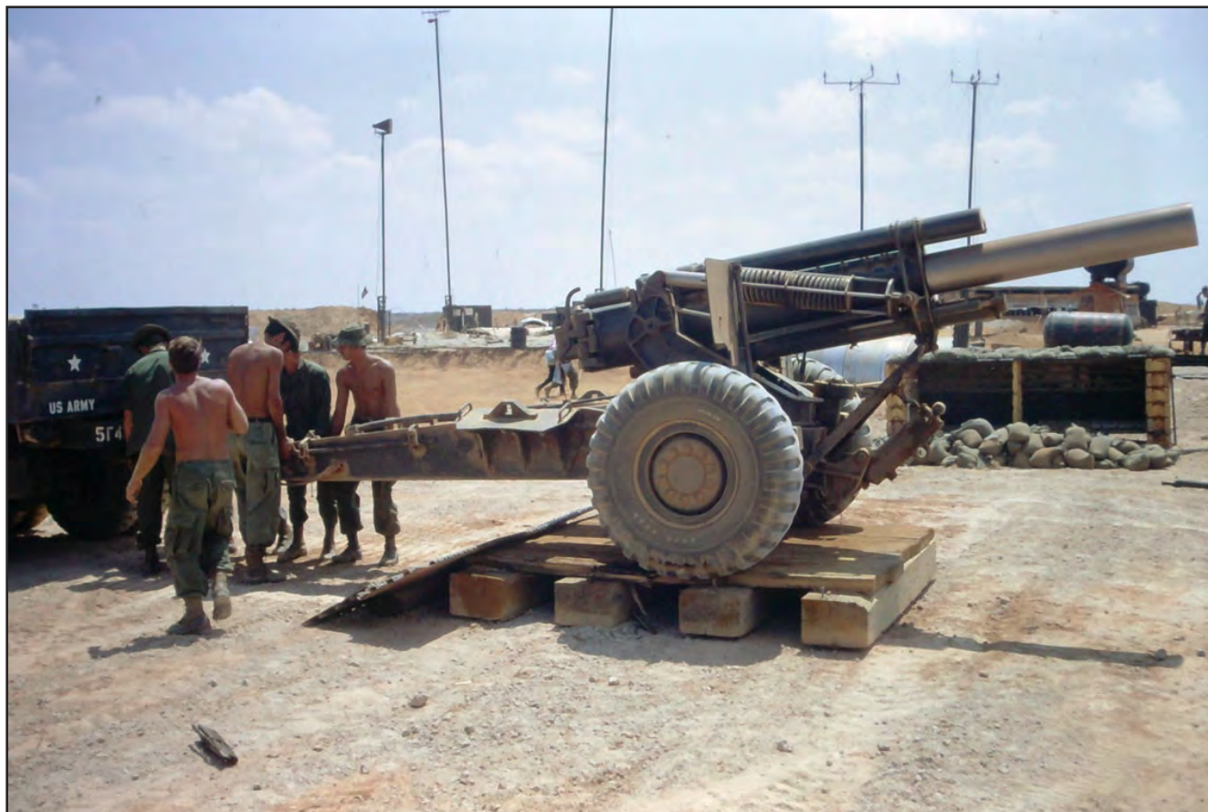
The howitzer is in place on the center of the platform. The men are unhooking the towing mechanism and preparing to spread the two trails from side to side.
