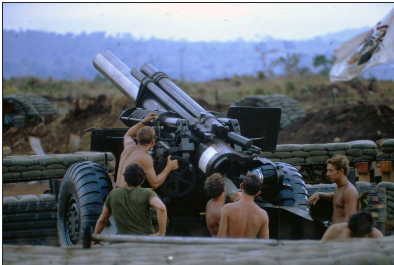
Preparing to fire a 155mm howitzer. The gunner is looking through the sight mounted on the left side of the howitzer. Another crew member is lifting a shell into the breech.
