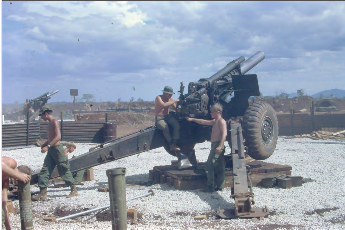
Preparing to fire a 155mm howitzer. The crew member on the right is holding the lanyard that triggered the firing pin. Another howitzer is seen to the left rear.
